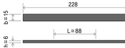
Fig. 1. Flexural test specimen dimension.
