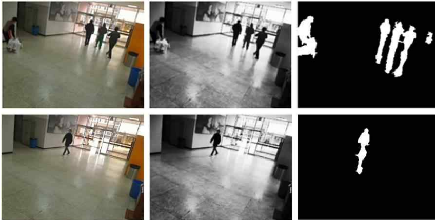
Fig. 3. The images having variations caused by light or shadow. Left figures: the original image. Middle figures: the gray image. Right figures: the segmented human areas having the reflection of the light or shadow.
