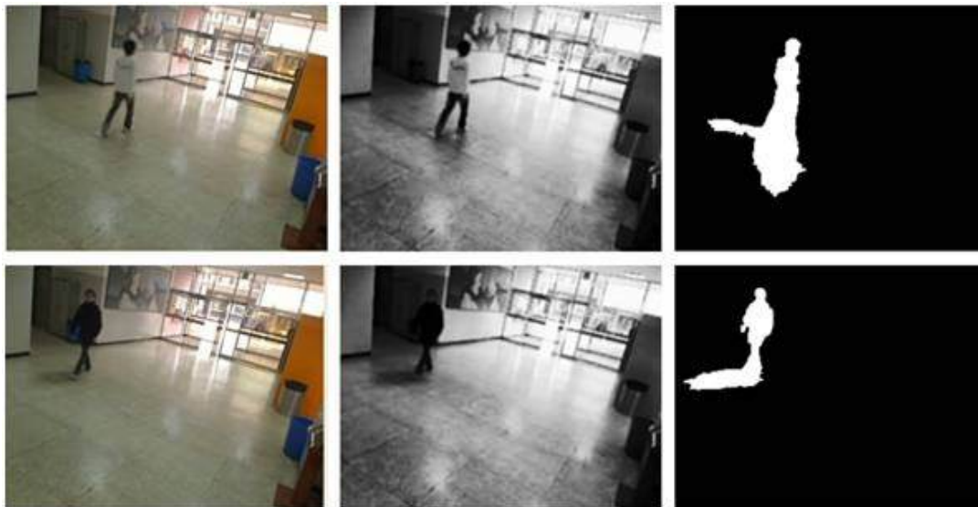
Fig. 2. The detection of the human area by the GMM. Left figures: the original image. Middle figures: the gray image. Right figures: the human area detected by using the GMM.
