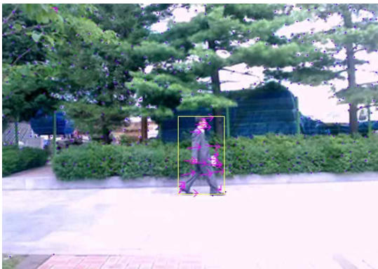
Fig. 7. The detected motion vectors by the LKT (points: the detected corner points by the LKT, arrows : the motion vectors calculated from the moved corner points in the successive images, box : the final box of human area).
