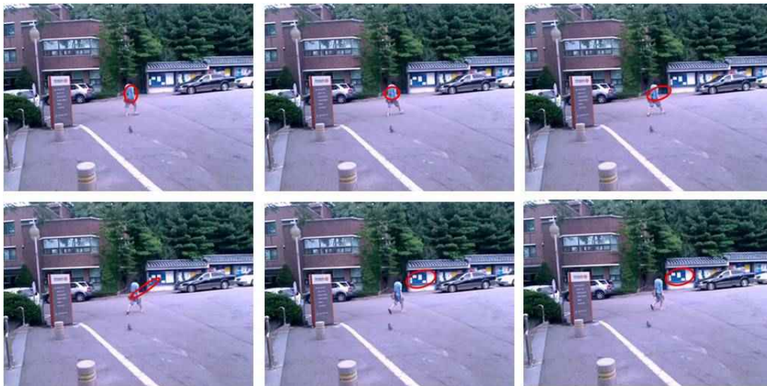
Fig. 15. the examples of false tracking result by the CamShift method with S3, S4 datasets.
