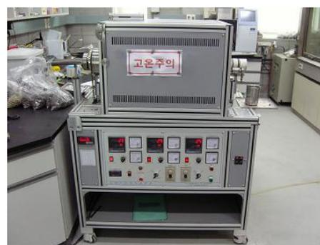
Fig. 2 Rotary tube furnace
