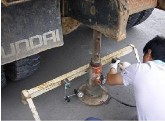
Fig. 6 View of the Plate Bearing Test
