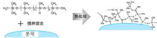
Fig. 24. Surface treatment of inorganic powder by polydimethylsiloxane (19) .
