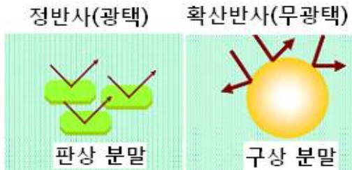
Fig. 5. The reflection of light from microsphere and platelet (2) .
