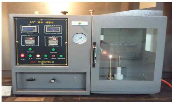
[Figure 3] Fire tester for flame propagation
