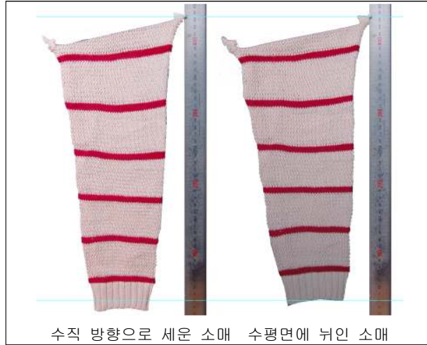
<Fig. 6> Actual longated arm part(left) due to its own weight
