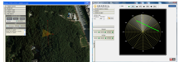
Fig. 7. Path of single moving target(left) and detected target path in radar(right)
