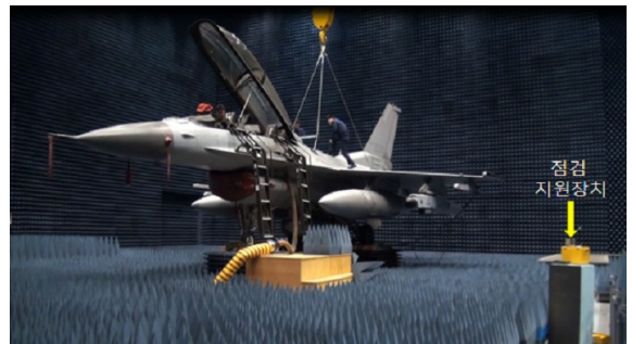
Fig. 13. Static Phase test(anechoic chamber)
