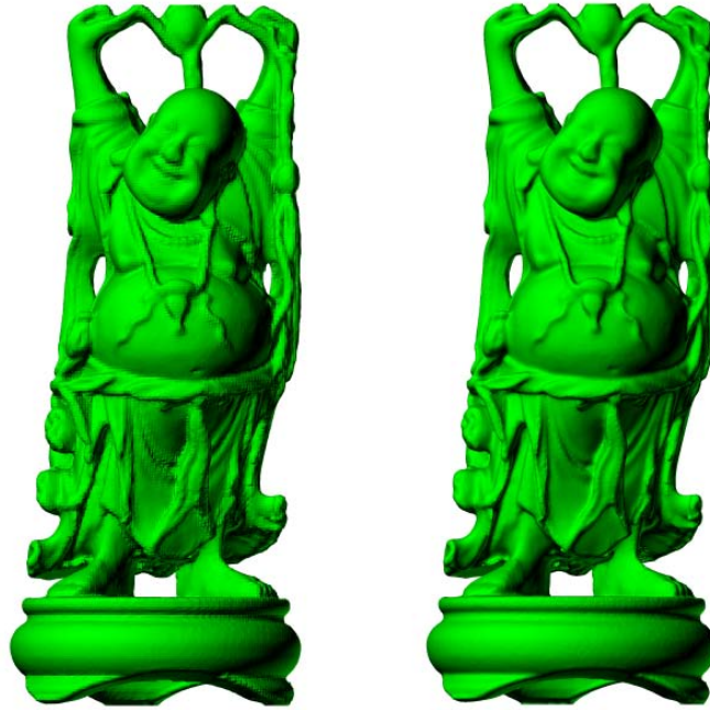
FIGURE 10. Three dimensional surface reconstruction for happy Buddha. The left one is acquired on the grid of which the maximum resolution is 256^3 and the right one does on the grid of 512^3 . The number of point is 543652.
