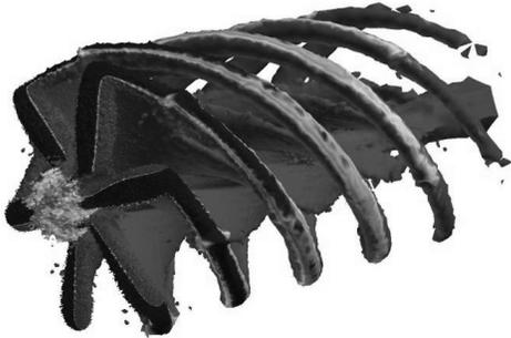
Fig. 11 Vorticity Distribution(Sliding Mesh)
