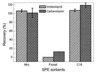
**Figure 5.** Recoveries of imidacloprid and carbendazim from spiked tomato samples with different SPE cartridges.
