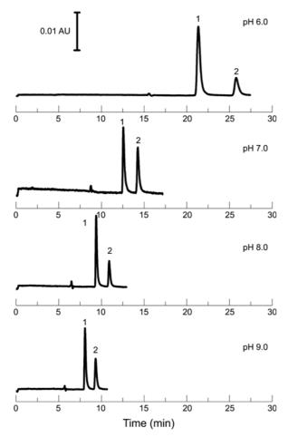
**Figure 3.** Effect of pH of running buffer on resolution. Mobile phase, 20 mmol·L<sup>-1</sup> phosphate buffer-acetonitrile (90:10, v/v); detection wavelength, 270 nm; applied voltage, 15 kV. Peak identification: 1, carbendazim; 2, imidacloprid.
