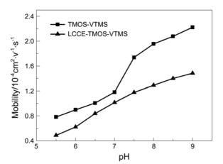
**Figure 2.** Effect of pH on EOF on the TMOS-VTMS and LCCE-TMOS-VTMS column. Buffer: 20 mmol·L<sup>-1</sup> phosphate buffer; EOF marker, thiourea; detection wavelength, 214 nm; applied voltage, 15 kV.
