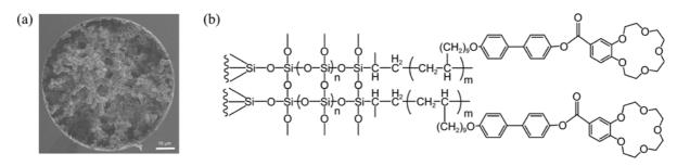
Figure 1. The scanning electron microscope image (a) and schematic (b) of LCCE-TMOS-VTMS column.
