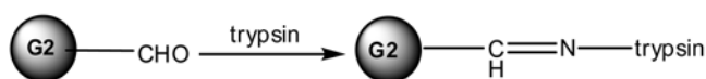
Figure 3. Enzyme Immobilization on aldehyde terminated dendrimer: stirring at 4 °C in phosphate buffer.
