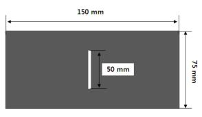
Fig. 4. The configuration of scribed coated specimens for undercutting evaluation.
