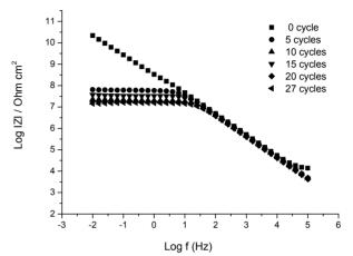
Fig. 12. EIS spectra for untreated epoxy coating with increasing hygrothermal cycles.
