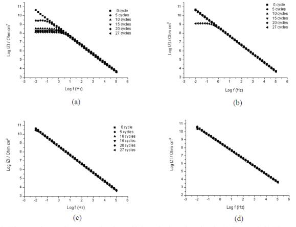
Fig. 13. EIS spectra for treated epoxy-coated surfaces with increasing hygrothermal cycle: (a) SB treated, (b) PT treated, (c) GS treated, and (d) GL treated.
