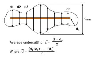
Fig. 5. Undercutting calculation based on Norsok standard M 501.
