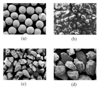
Fig. 2. SEM images of abrasives used in this study: (a) steel shot ball, (b) grinder wheel, (c) steel grit with 0.4 mm diameter and (d) steel grit with 0.8 mm diameter.
