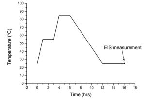
Fig. 6. Heating cycle used in the hygrothermal cyclic test.
