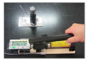
Fig. 3. Pull-off adhesion test equipment.
