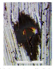
**Fig. 14.** Optical microscopy image of localized corrosion at the epoxy coat/carbon steel interface of PT treated steel after 27 cycles of hygrothermal testing.
