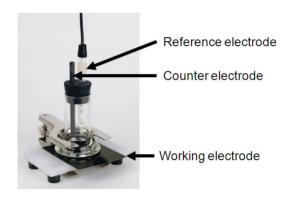
Fig. 7. Three-electrode electrochemical cell for EIS tests.
