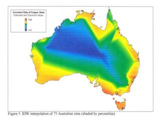
Fig. 2. Corrosion map of Australia by IDW model.
