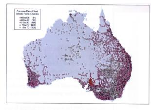
Corrosion rate of steel in selected towns in Australia
