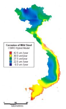
Fig. 4. Corrosion map of Viet nam by IDW Model.
