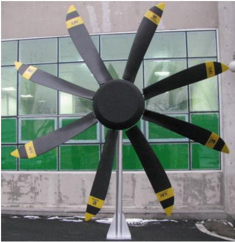
Fig. 19 View of prototype propeller assembly with 8 blades
