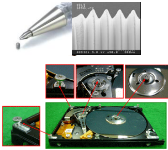
Fig. 1 General application of micro screw in HDD
