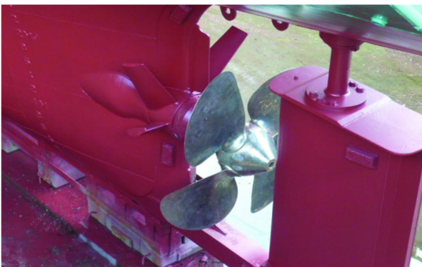
Fig. 4 New pre-swirl stator "Eco-stator"
