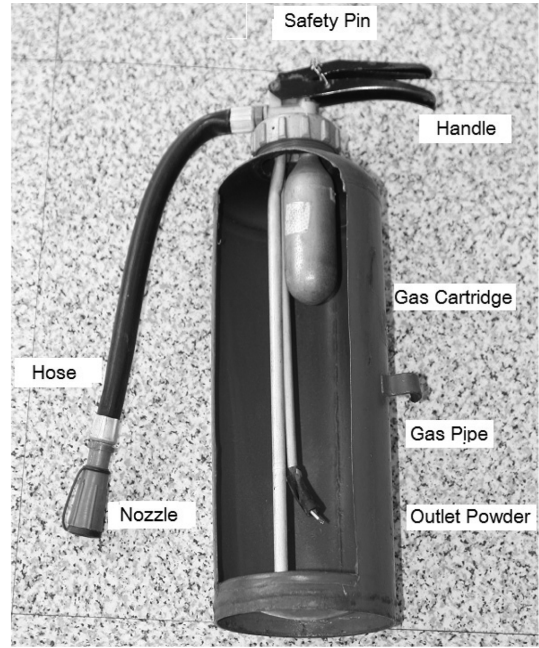
Figure 2. View of cut gas cartridge type fire extinguisher.
