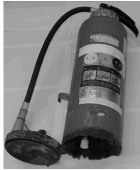
Figure 1. Exploded fire extinguisher of case 4 (10) .
