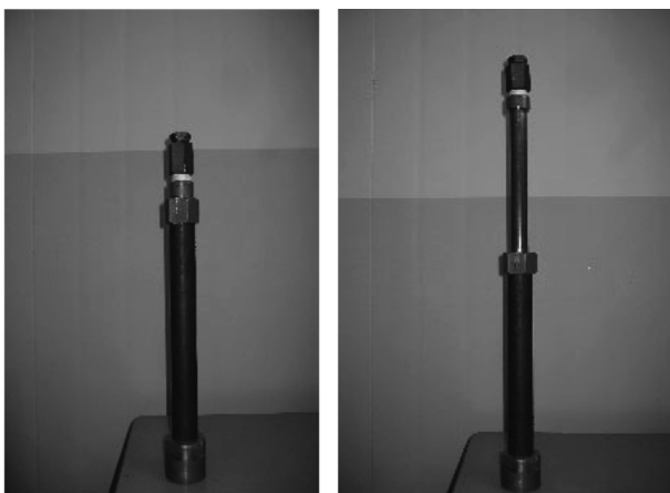
Figure 2. Before and after Photos of operation of water curtain nozzles.
