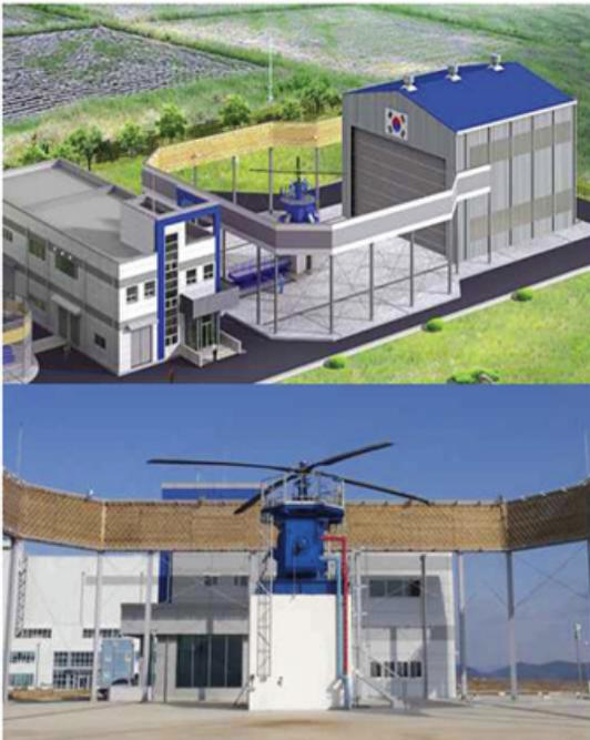
Fig. 1 Whirl Tower Test Facility
