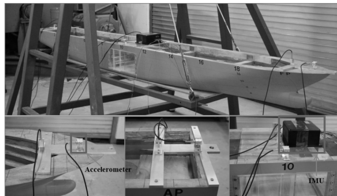
Fig. 3 Motion measurement system (IMU &amp; accelerometers).
