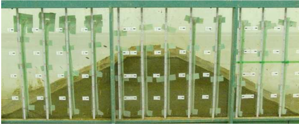
(a) The Levee Model Constructed (Case-1)
