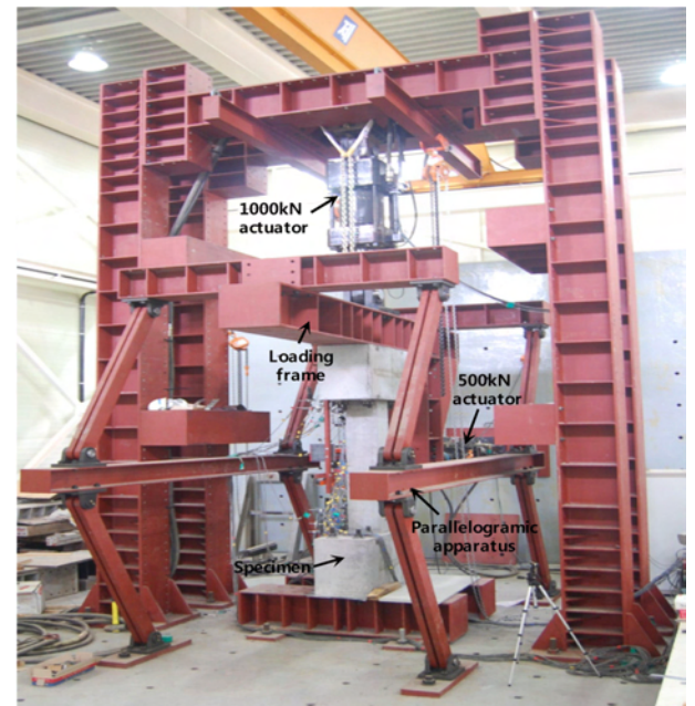
Fig. 3 Test setup of specimens
