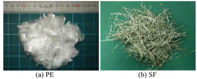
Fig. 1 Shapes of fibers
