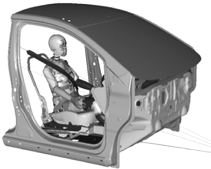
Fig. 2 Belt fitting for crash simulation
