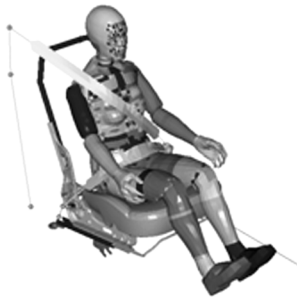
Fig. 1 Modeling of a safety belt system for crash simulation
