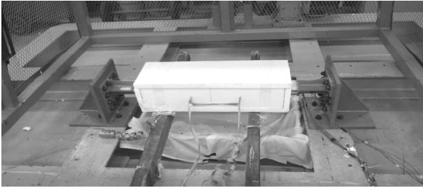
Fig. 4 Model installed at drop test bed
