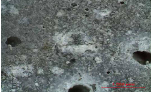
Fig. 4. Cracking on slate mortar bar with 10% flyash
