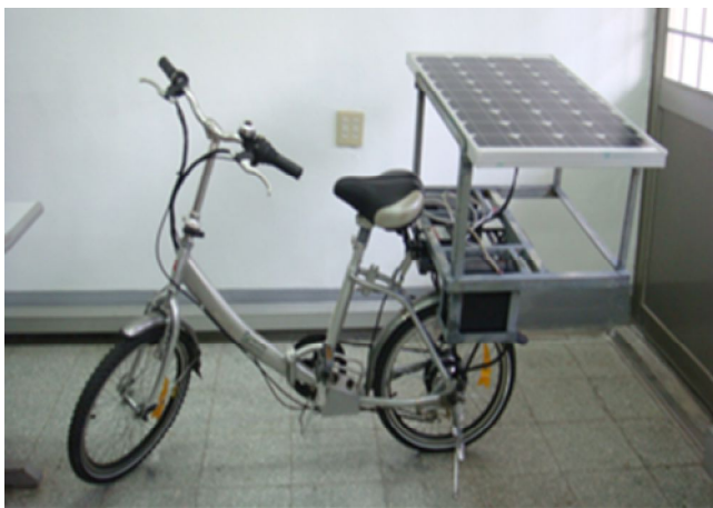
Fig. 1. Prototype of the proposed solar energy powered bicycle
