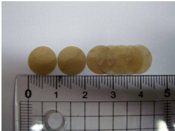
Fig. 3. Picture of PPLP sample used for measurement.
