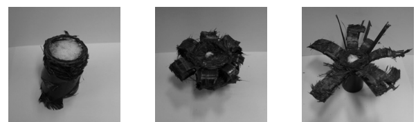
(1) CFRP/Foam circular member according to stacking angle, Foam density(40)
