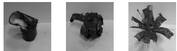
(2) CFRP/Foam circular member according to stacking angle, Foam density(60)
