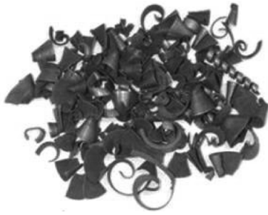
Fig. 1. Zero-valent iron from waste steel scrap.
