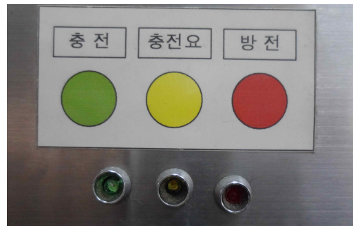
Photo 3. LED indication lamp for battery charging state.
