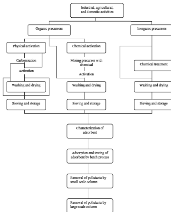
Fig. 1. Protocol for development of low-cost adsorbents and their utilization for wastewater treatment. 4)
