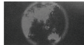
Figure 4 (excerpt from [10]) Optical reconstruction of the hologram of a globe image generated with the IWRP method
