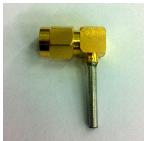
Fig. 3 Coaxial line sensor (a) dimension and materials of coaxial line and (b) photograph of manufactured sensor
