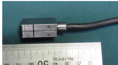
Fig. 6 Shear wave phased array ultrasonic probe
