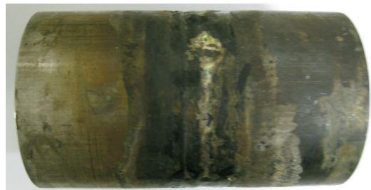
(b) DMW defect specimen
