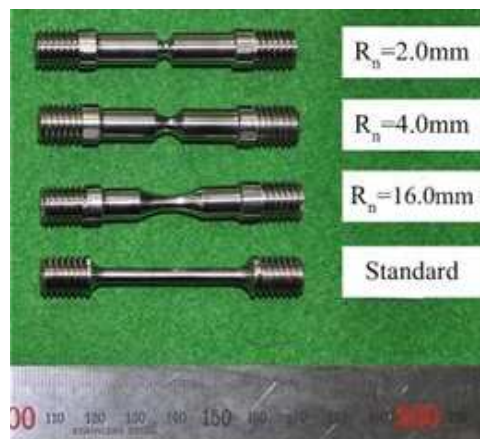
Fig. 2 Tensile specimens with various notch radius
