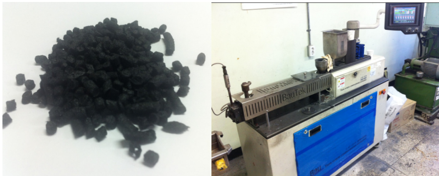
Figure 7. Pellets extruded from the 2-axis extruder.
