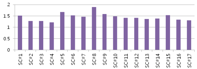
Figure 12. Specific gravity of various rubber composites for synthetic turf filler.
