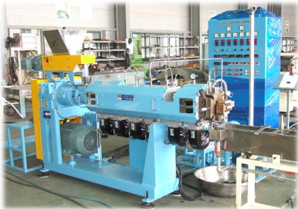
Figure 10. The continuous supercritical fluid extruder.
