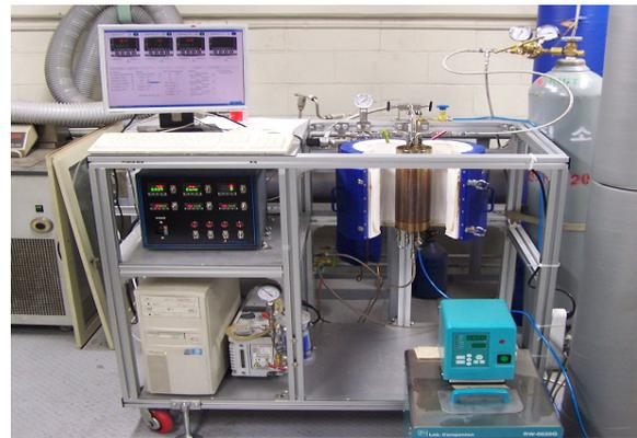
Figure 8. The batch type of supercritical reactor.
