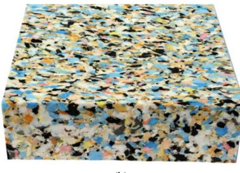
**Figure 1.** Process for the rebonded foam from flexible PU foam scraps (a) and a photograph of the rebonded foam (b).
