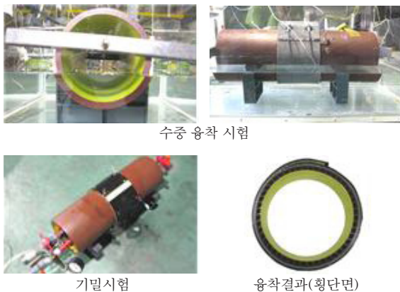
Fig. 15. Fusion under submerged condition, (Pressure= 0.1 MPa)
