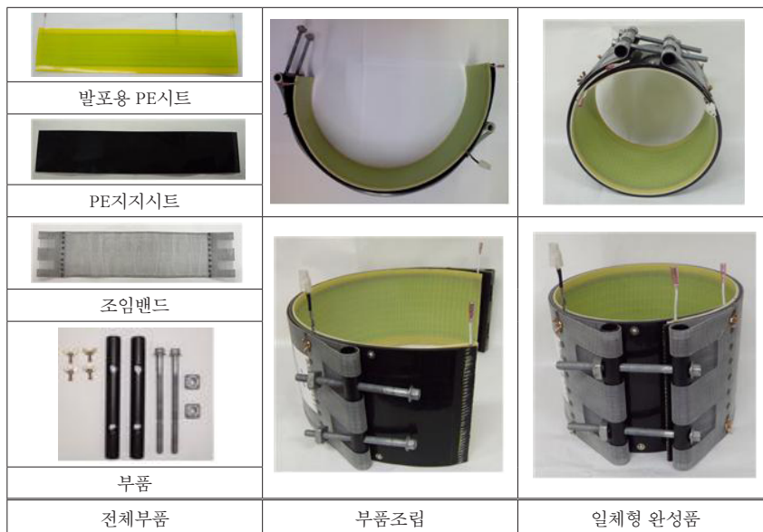
Fig. 10. All in one assembly of EFF fitting.
