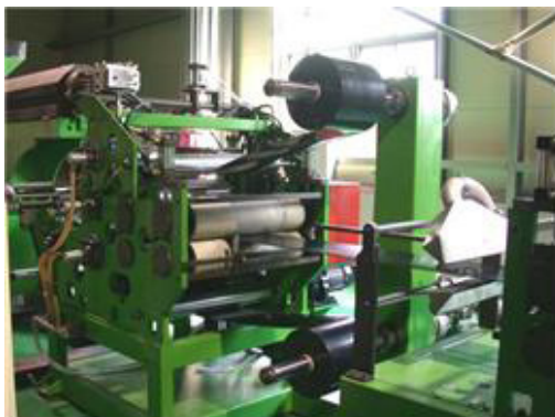
Fig. 7. Casting roll mill.
