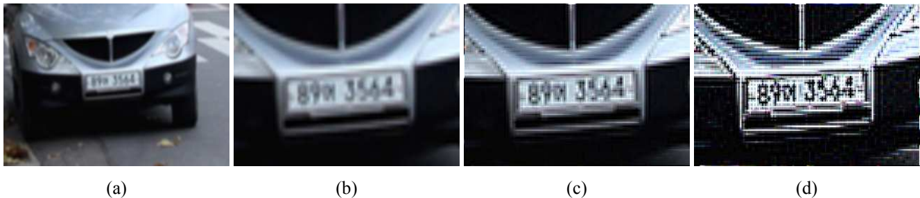
Fig. 4. The super-resolution method results: (a) the low-resolution input image, (b) the upsampled image using bilinear interpolation, (c) the visually optimized result of spatially adaptive super-resolution, and (d) the spatially adaptive super-resolution result used for license plate recognition
