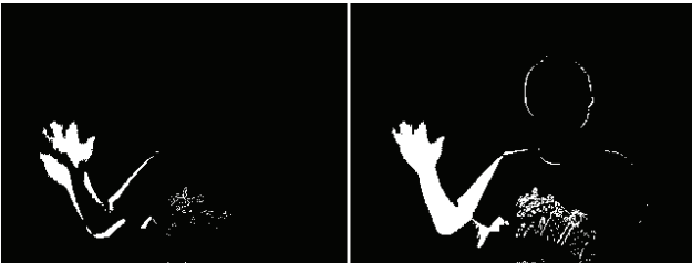
Fig. 3. Comparisons of pixel-based moving object detection algorithms when n=14 . The left image is the result of the simple difference image, and the right image is the result of the frame voting algorithm.
