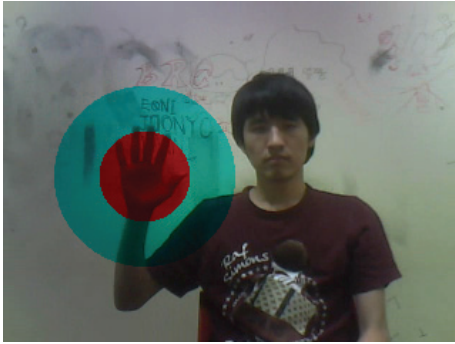
Fig. 5. The region of interest (ROI, red circle) and adjacent background region (ABR, green donut).
