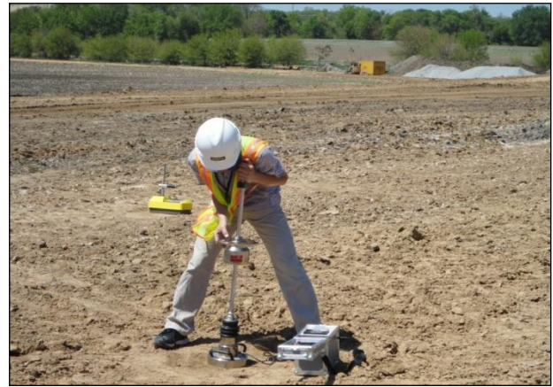
FIGURE IV MEASURING STIFFNESS OF THE SOIL WITH THE LWD
