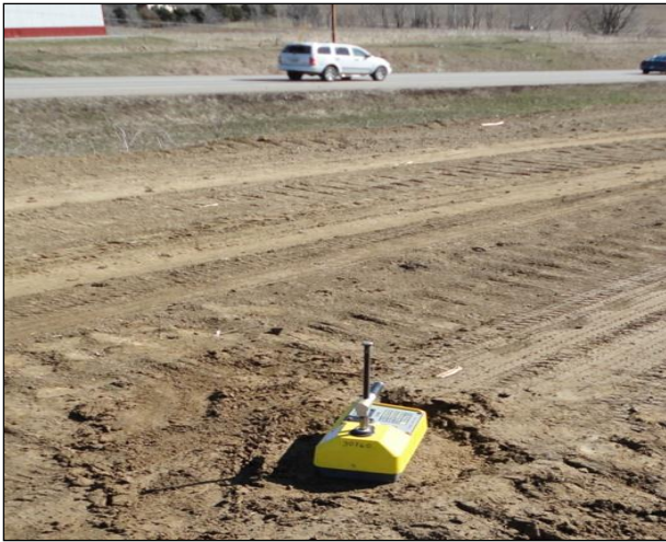
FIGURE II NUCLEAR GAUGE TAKING SOIL MEASUREMENTS
