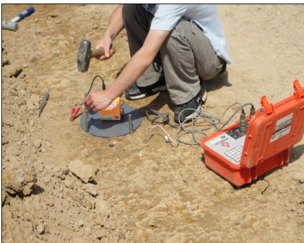
FIGURE III DARTS DRIVEN INTO GROUND FOR EDG TEST
