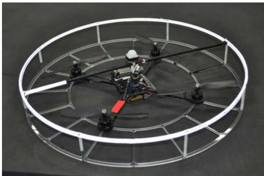
Figure 4: Quadrotor-type vehicle equipped with the proposed circular ring pattern.
