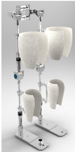
Figure 7: Design of the exoskeleton
