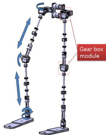
Figure 6: Joint structure of exoskeleton
