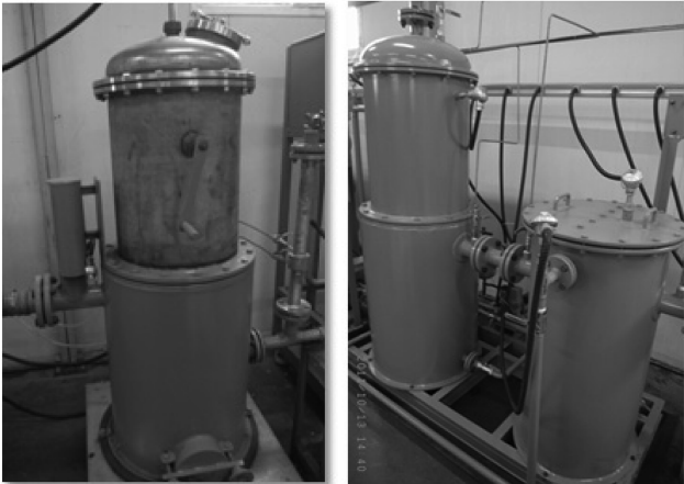
Fig. 2 Downdraft gasifier (left) and hot filter before water scrubber (right)
