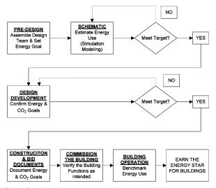
(Fig. 1) Incorporating energy targets, analysis, and tracking during design and operating phases of the building (modified from the EPA Energy Design Guidance) [13]
